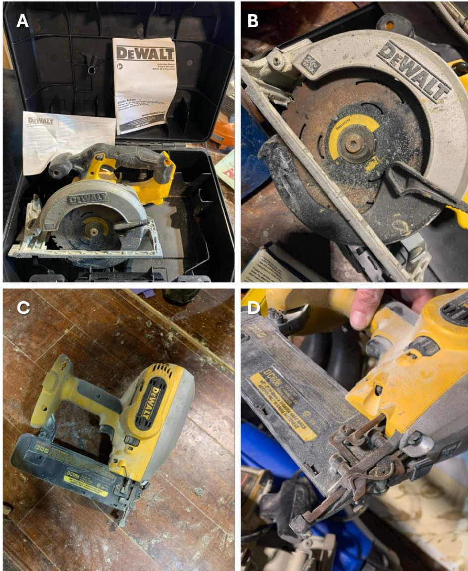
Figure 1: Corrosion of homeowners' tools. (A) DeWalt Circular Saw, one day after the fire event, no corrosion is evident. (B) DeWalt Circular Saw, one week after the fire event, new corrosion is evident. (C) DeWalt Brad Nailer, one day after the fire event, no corrosion is evident. (D) DeWalt Brad Nailer, one week after the fire event, new corrosion is evident.
